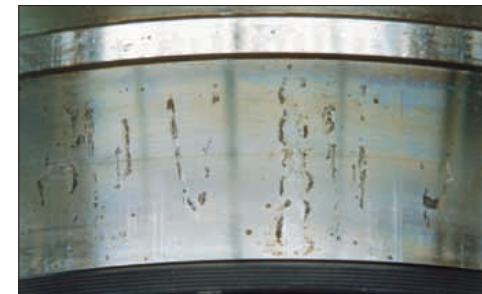
Photo 16-3 Part: Inner ring of a spherical roller bearing Symptom: Rust on raceway surface at roller pitch Cause: Entry of water into lubricant
