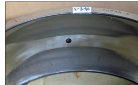
Photo 10-3 Part: Outer ring of a spherical roller bearing Symptom: Wear occurs on loaded side of raceway surface Cause: Low speed, heavy load and poor lubrication (No oil film)
