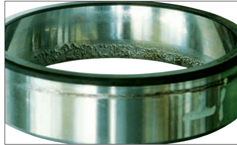
Photo 1-6 Part: Outer ring of Photo 1-5 Symptom: Flaking of only one raceway over its entire circumference Cause: Excessive axial load
