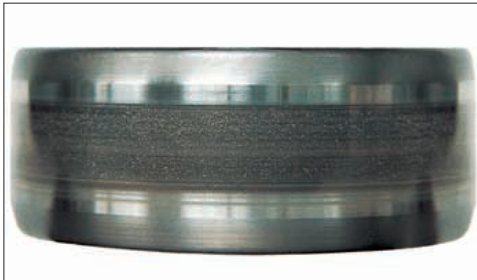
Photo 15-3 Part: Inner ring of a cylindrical roller bearing Symptom: Belt pattern of electrical corrosion accompanied by pits on the raceway surface
