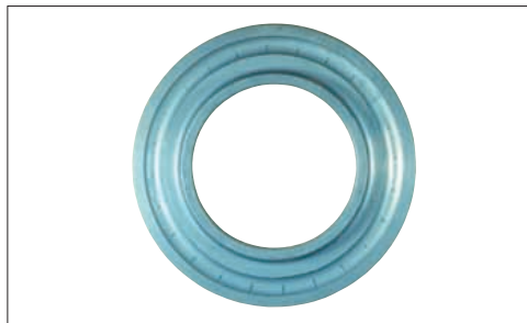
Photo 12-3 Part: Outer ring of a thrust ball bearing Symptom: False brinelling of raceway surface at ball pitch Cause: Repeated vibration with a small oscillating angle
