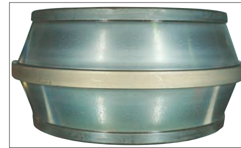
Photo 8-1 Part: Inner ring of a double-row tapered roller bearing Symptom: Frosted raceway surface Cause: Debris caught in the surface
