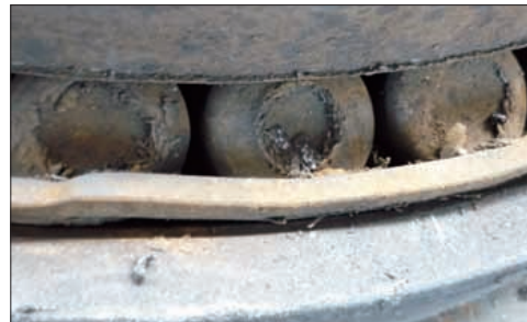
Photo 13-6 Part: Rollers of a large tapered roller bearing Symptom: Seizure occur at large end face of roller Cause: Poor lubrication and excessive axial load
