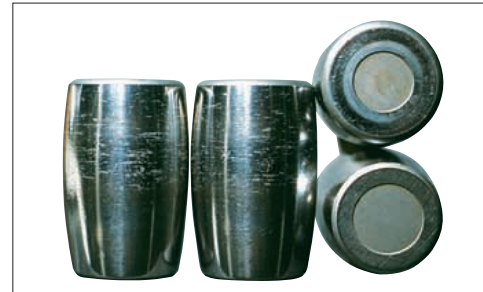
Photo 3-2 Part: Convex rollers of Photo 3-1 Symptom: Scoring on roller end face Cause: Roller slipping due to sudden acceleration and deceleration
