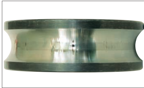
Photo 12-1 Part: Inner ring of a deep groove ball bearing Symptom: False brinelling occurs on the raceway Cause: Vibration from an external source while stationary
