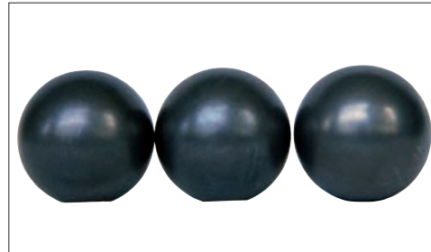
Photo 15-4 Part: Balls of a groove ball bearing Symptom: Electrical corrosion has a dark color that covers the entire ball surface
