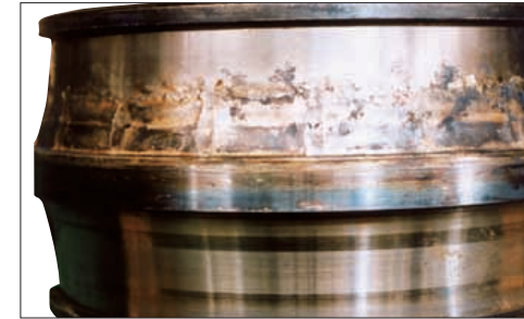
Photo 13-1 Part: Inner ring of a spherical roller bearing Symptom: Raceway is discolored and melted. Worn particles from the cage were rolled and attached to the raceway Cause: Insufficient lubrication
