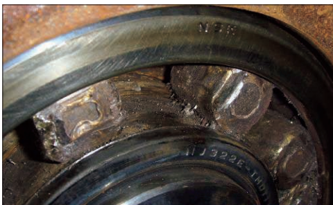
Photo 13-7 Part: Cylindrical roller bearing Symptom: Seizure occurs on ring raceway surface and roller Cause: Excessively small internal clearance causes heat generation by sliding of the inner ring and rollers under high speed and light load
