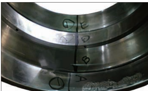
Photo 1-9 Part: Outer ring of a four-row tapered roller bearing Symptom: Flaking of raceway (Loading area) Cause: Excessive moment load
