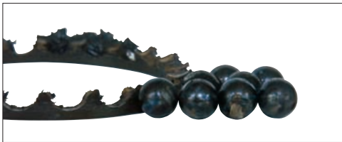
Photo 13-5 Part: Balls and cage of Photo 13-3 Symptom: Cage is damaged by melting, balls become discolored and melted Cause: Excessive preload
