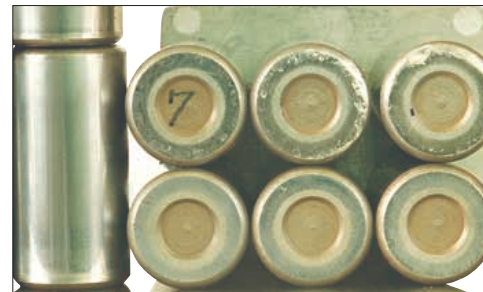
Photo 3-4 Part: Rollers of a double-row cylindrical roller bearing Symptom: Scoring on the roller end face Cause: Poor lubrication and excessive axial load
