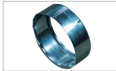
Photo 5-4 Part: Outer ring of a solid type needle roller bearing Symptom: Fracture occurs at the outer ring rib Roller inclination due to excessive loading (Needle rollers are long compared to their diameter. Under excessive or uneven loading, rollers become inclined and push against the ribs.) Cause:
