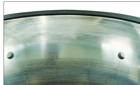
Photo 4-4 Part: Outer ring of Photo 4-3 Symptom: Smearing occurs circumferentially on raceway surface Cause: Poor lubrication
