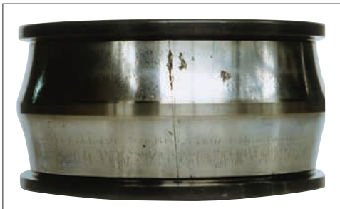
Photo 6-6 Part: Inner ring of a spherical roller bearing Symptom: Axial cracks occur on raceway surface Cause: Large fitting stress due to temperature difference between shaft and inner ring
