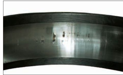
Photo 12-2 Part: Outer ring of Photo 12-1 Symptom: False brinelling occurs on the raceway Cause: Vibration from an external source while stationary
