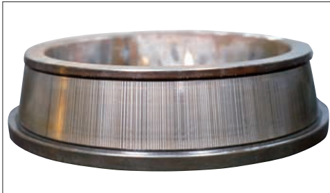
Photo 15-1 Part: Inner ring of a tapered roller bearing Symptom: Striped pattern of corrosion occurs on the raceway surface
