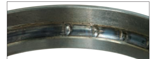
Photo 13-4 Part: Outer ring in Photo 13-3 Symptom: Raceway discoloration, melting occurs at ball pitch intervals Cause: Excessive preload
