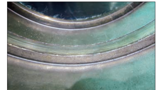
Photo 3-8 Part: Outer ring of a double-row cylindrical roller bearing Symptom: Notable scoring on the face of outer ring rib Cause: Excessive axial loading
