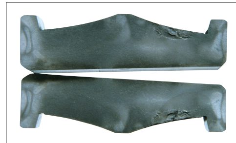
Photo 6-7 Part: Cross section of a fractured inner ring in Photo 6-6 Symptom: Origin is directly beneath the raceway surface
