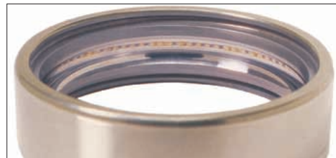
Photo 15-6 Part: Outer ring of a deep groove ball bearing Symptom: Fluting occurs on the raceway surface (High frequency)
