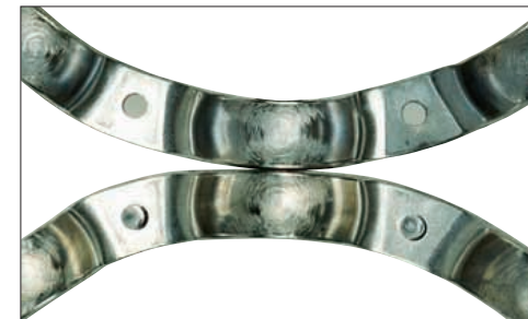
Photo 3-7 Part: Cage of a deep groove ball bearing Symptom: Scoring on the pressed-steel cage pockets Cause: Entry of debris
