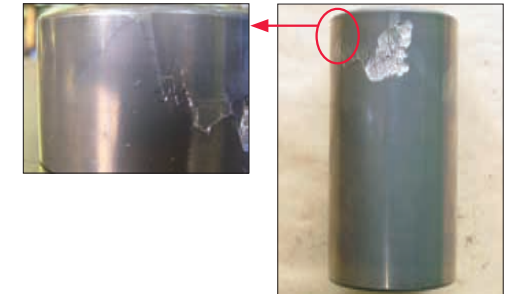
Photo 1-14 Part: Roller of a cylindrical roller bearing Symptom: Flaking of rolling surfaces Cause: Origin from flaw or crack in roller during mounting of outer ring and roller
