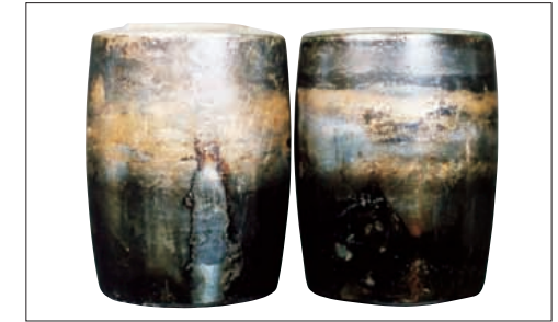
Photo 13-2 Part: Convex rollers of Photo 13-1 Symptom: Discoloration and melting of roller rolling surface, adhesion of worn particles from cage Cause: Insufficient lubrication
