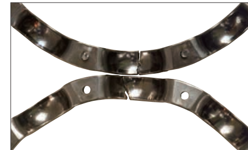
Photo 7-1 Part: Cage of a deep groove ball bearing Symptom: Fracture of pressed-steel cage-pocket
