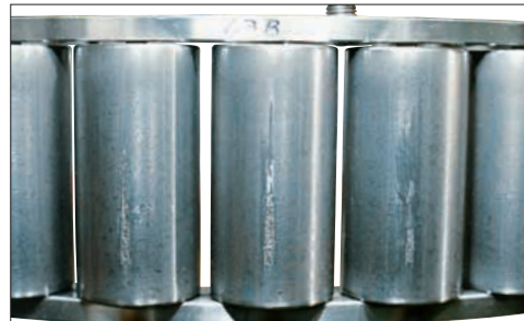
Photo 1-8 Part: Rollers of a cylindrical roller bearing Symptom: Premature flaking occurs axially on the rolling surfaces Cause: Scratches caused during improper mounting
