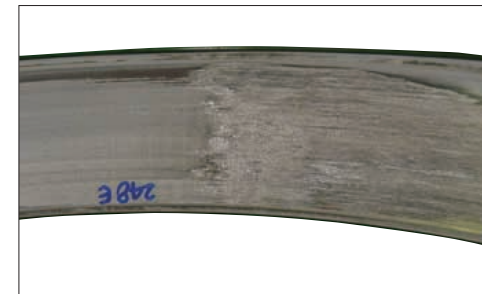
Photo 4-9 Part: Outer ring of a large tapered roller bearing Symptom: Smearing occurs on outer ring raceway surface Cause: High speed, light load and poor lubrication
