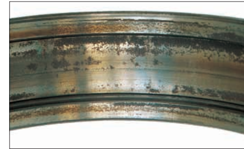
Photo 16-1 Part: Outer ring of a cylindrical roller bearing Symptom: Rust on the rib face and raceway surface Cause: Poor lubrication due to water entry
