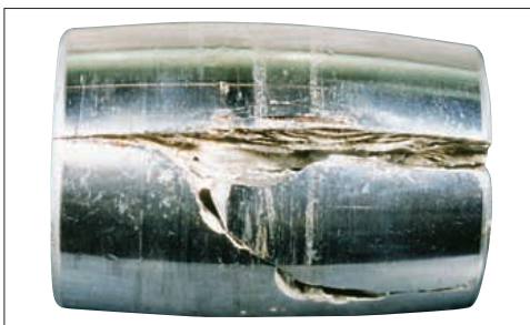
Photo 6-8 Part: Roller of a spherical roller bearing Symptom: Axial cracks occur on rolling surface
