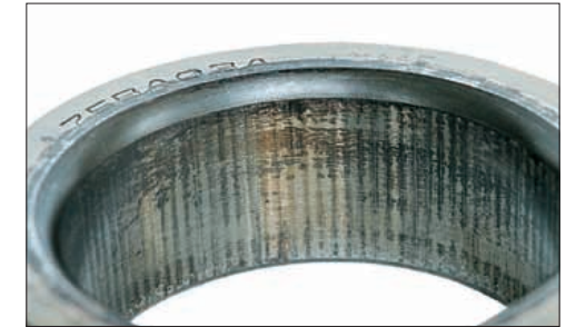
Photo 11-2 Part: Inner ring of an angular contact ball bearing Symptom: Notable fretting occurs over entire circumference of bore surface Cause: Insufficient interference fit
