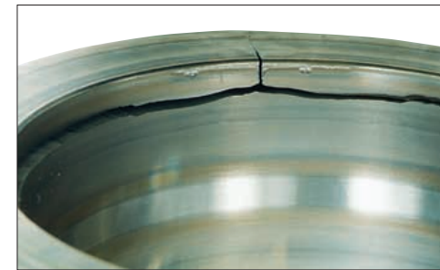
Photo 6-3 Part: Outer ring of a double-row cylindrical roller bearing Symptom: Cracks propagated outward in the axial and circumferential directions from the flaking origin on the raceway surface Cause: Flaking from a flaw due to shock
