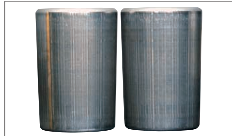
Photo 15-2 Part: Tapered rollers in Photo 15-1 Symptom: Striped pattern of corrosion occurs on the rolling surface
