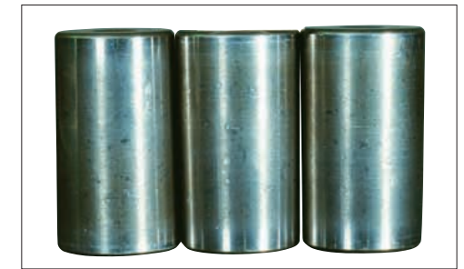
Photo 8-4 Part: Tapered rollers of Photo 8-3 Symptom: Small and large indentations occur over the rolling surface Cause: Debris caught in the surface
