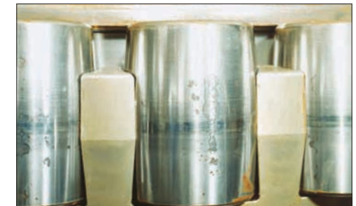
Photo 16-4 Part: Rollers of a spherical roller bearing Symptom: Pit-shaped rust on rolling contact surface. Corroded portions. Cause: Moisture condensation during storage
