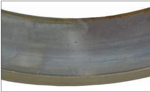
Photo 10-5 Part: Outer ring of a tapered roller bearing Symptom: Wear occurs on outer ring raceway surface Cause: Insufficient oil film and wear due to poor lubrication
