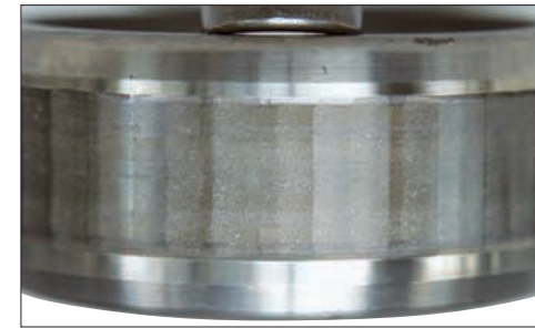
Photo 10-1 Part: Inner ring of a cylindrical roller bearing Symptom: Many pits occur due to electrical corrosion and wave-shaped wear on raceway surface Cause: Electrical corrosion
