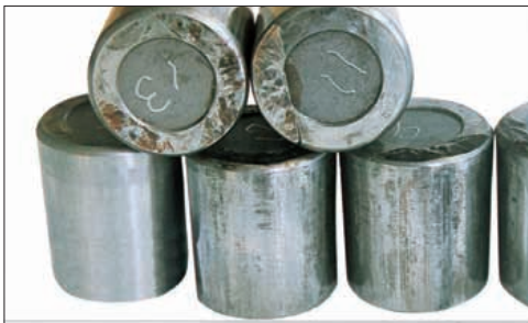
Photo 10-7 Part: Tapered rollers of Photo 10-6 Symptom: Stepped wear on the roller head and face Cause: Fretting progression due to excessive load while stationary
