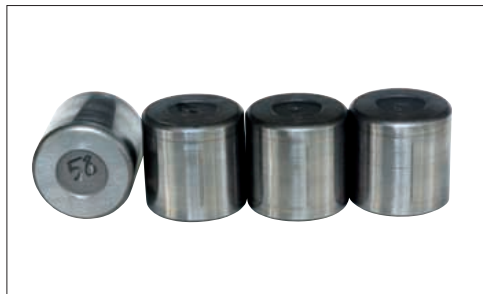
Photo 17-3 Part: Rollers of a cylindrical roller bearing Symptom: Axial scratches on rolling surface Cause: Inclination of inner and outer rings during mounting
