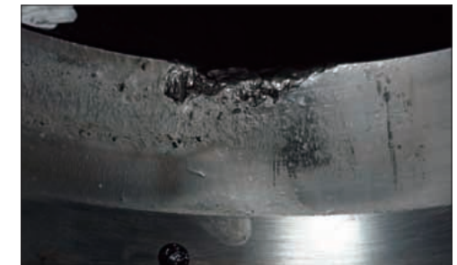
Photo 10-4 Part: Outer ring of a spherical roller bearing (enlargement) Symptom: Example of small flaking and wear combined on the raceway Cause: Insufficient oil film due to poor lubrication leads to wear (primary damage) that progresses to flaking (secondary damage)
