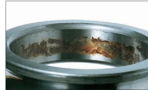
Photo 11-1 Part: Inner ring of a deep groove ball bearing Symptom: Fretting occurs on the bore surface Cause: Vibration
