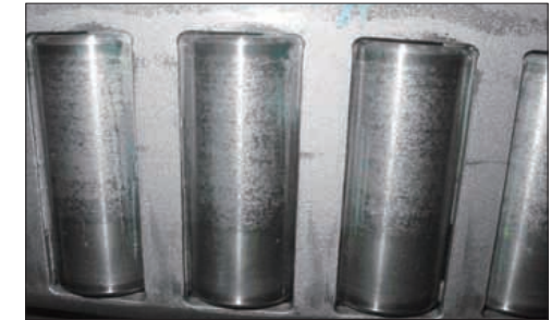
Photo 4-8 Part: Rollers of a large cylindrical roller bearing Symptom: Smearing occurs on rolling surface Cause: Light load and poor lubrication
