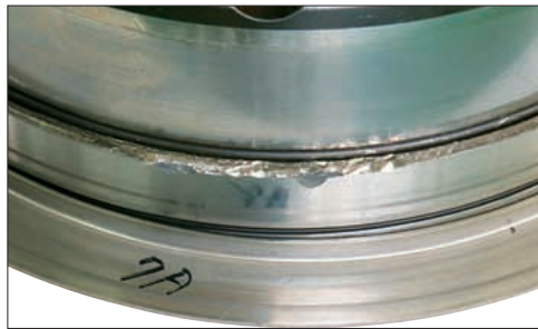
Photo 5-1 Part: Inner ring of a double-row cylindrical roller bearing Symptom: Chipping occurs at the center rib Cause: Excessive load during mounting
