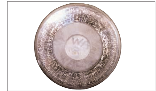
Photo 6-2 Part: Roller of a tapered roller thrust bearing Symptom: Thermal cracks occur at large end face of roller Cause: Heat generation due to sliding with the inner ring rib under poor lubrication
